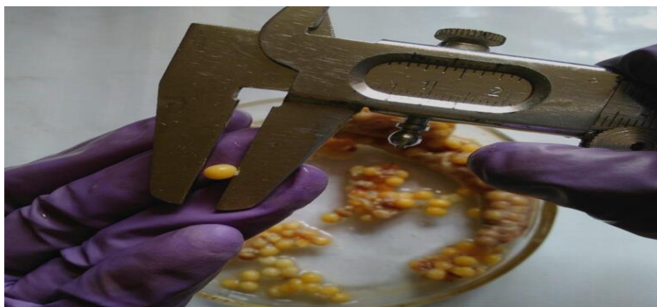
Fig-4(c): Measurement of Ova diameter using Slide Callipers
